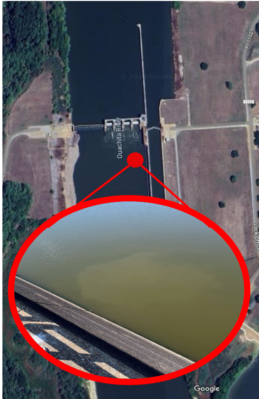
Water changes indicate that the boil location is outside of the lock chamber
